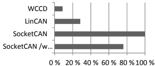
Figure 6. Measured CPU load when transmitting 1000 frames/s.
