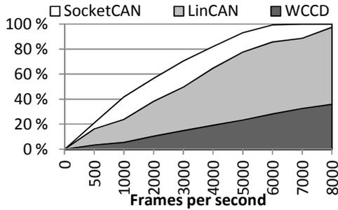
Figure 3. CPU load on receive.
