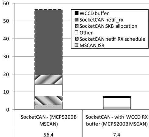
Figure 7. CAN receive ISR execution time (us). Tasks listed in execution order (earliest at bottom).
