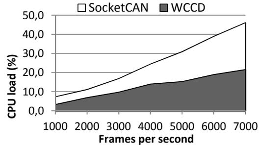
Figure 8. CPU load on CAN receive, PowerPC platform.
