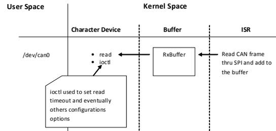
Figure 1. Receive buffer implementation.
