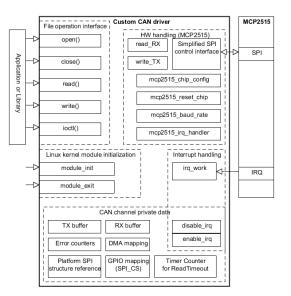
Figure 2. WCCD architecture on ARM platform using an external SPI CAN-controller (MPC2515).
