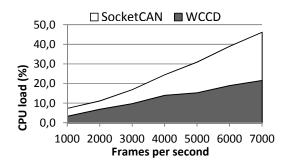
Figure 8. CPU load on CAN receive, PowerPC platform.
