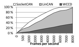
Figure 3. CPU load on receive.
