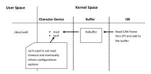
Figure 1. Receive buffer implementation.
